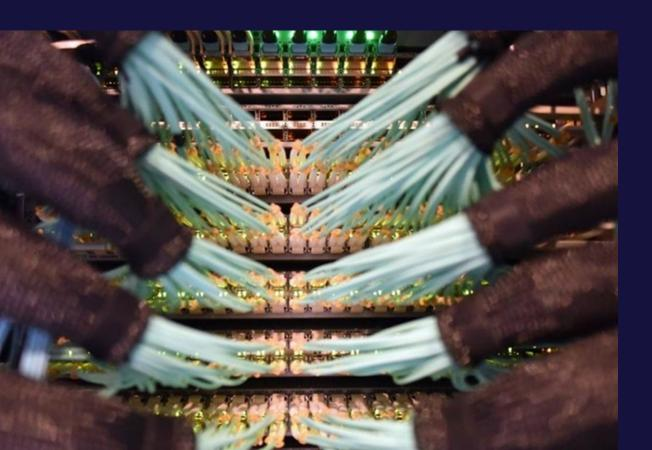
These fibers with 10/40G transceivers carry 100% of the signals necessary to support one 32 camera UHD OB truck, with twelve replay servers and multi-viewing for almost 500 unique sources
