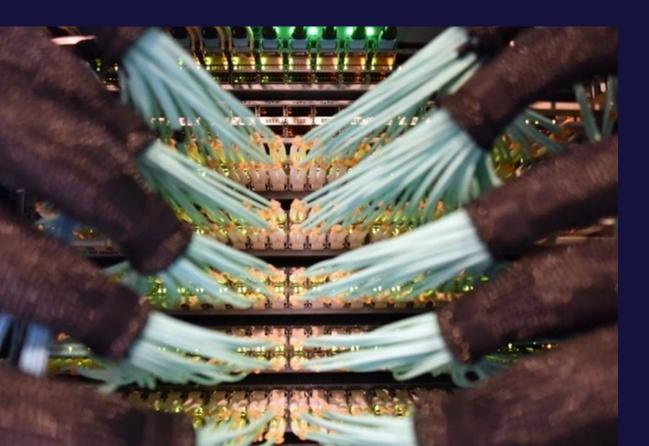
These fibers with 10/40G transceivers carry 100% of the signals necessary to support one 32 camera UHD OB truck, with twelve replay servers and multi-viewing for almost 500 unique sources
