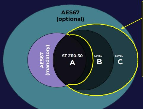
These two operating points (ST 2110-30 Level B & Level C) both support a shorter packet time of **125** μSEC, ideal for low-latency LIVE PRODUCTION
